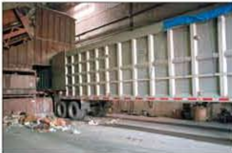
Unloader® Live-Floor/Compactor Compatible Trailer – Designed with reinforced bulkhead and side wall bracing to handle compactor loading forces.
