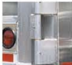
Greaseable extruded hinge. Designed for longer life, low maintenance.
