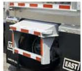
Subframe integrated with push block.
