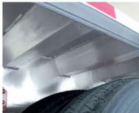
Aerodynamic V-shaped cross-members.
