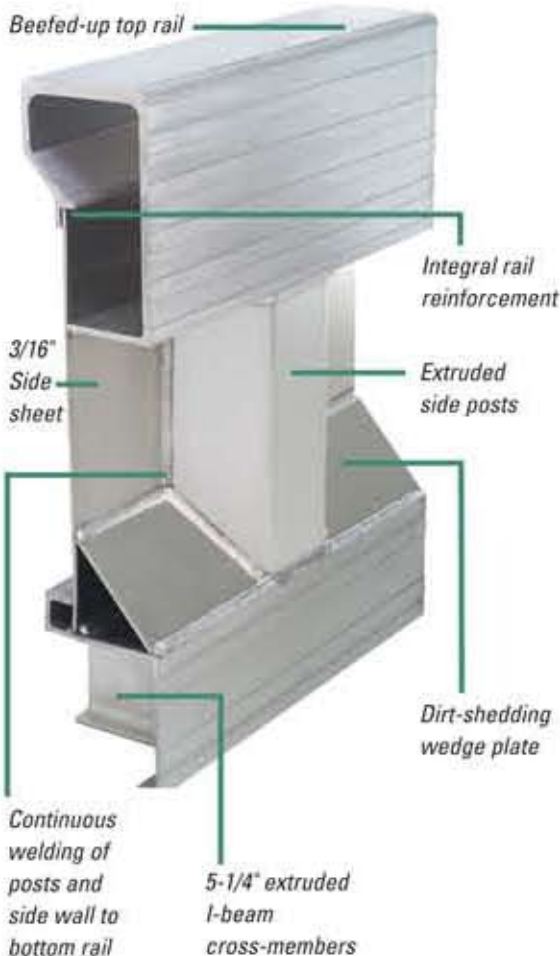
Stronger floor construction.
