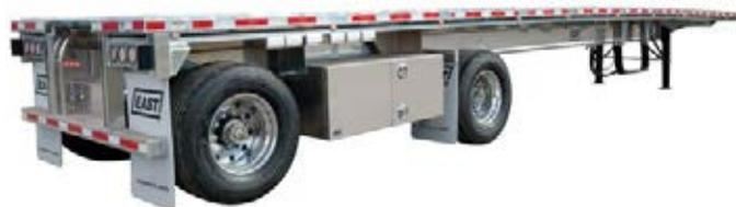
**BEAST™ II (BST II)** – Designed with all the features and benefits of the Beast, the Beast II meets the needs of applications requiring higher concentrated load ratings without additional weight. It handles loads up to 65,000 lbs. concentrated in 4 feet on a 48-foot wide-spread tandem-axle trailer and up to 100,000 lbs. distributed. Ideal for two to three-axle configurations, it is available in lengths up to 53 feet and boasts a 13-inch neck with a 2-inch deeper main beam than the BST.
