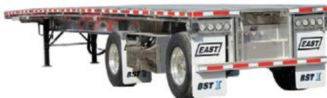
**MMX™** – Offering one of the highest concentrated load ratings in an aluminum flatbed, the MMX is rated to handle loads up to 80,000 lbs. concentrated in 4 feet on a 48-foot wide-spread trailer, and up to 145,000 lbs. with a multi-axle configuration. Ideal for multi-axle applications, it is available in lengths up to 53 feet and boasts a 12½-inch deep neck with a super-duty main beam.
